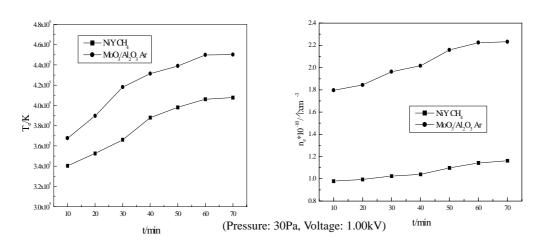
Figure 1 Electron temperature *versus* time
